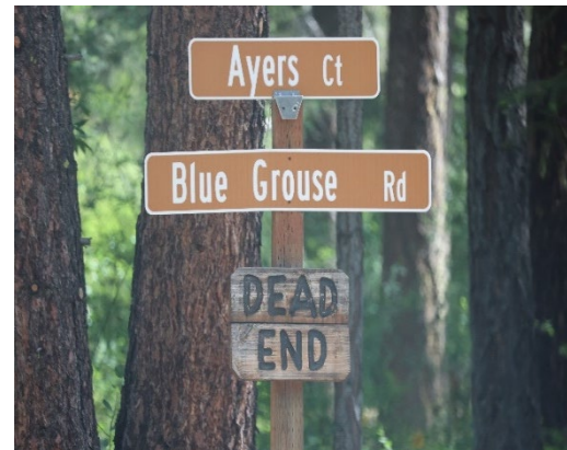
Figure 1.b.11. Address and road signage across the county is not cohesive and varies vastly in quality and utility. In this example the road signage is sufficient, but the non-reflective "DEAD END" sign would not be easily visible to first responders and firefighters during an emergency wildfire event. (Source: Eli Loftis, Okanogan CD, 2024)
