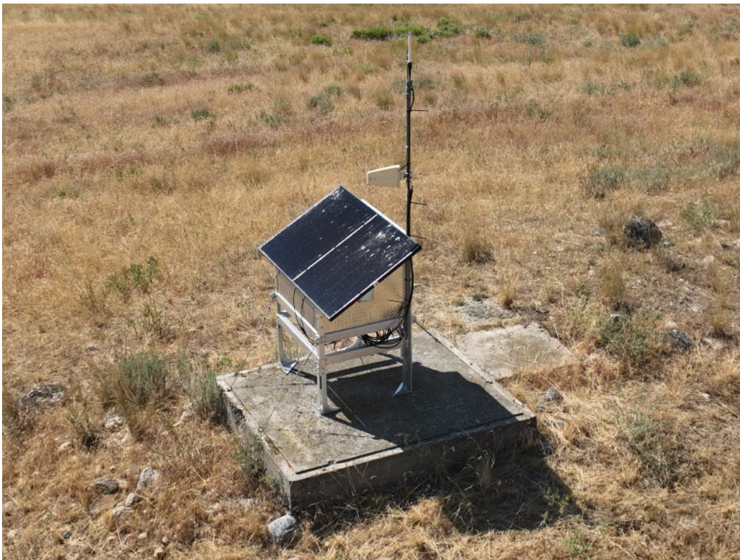
Figure E.3 An emerging technology, virtual fencing has the dual benefit of reducing the need for physical fences that are vulnerable to fire damage, and removing barriers for wildlife such as pronghorn and grouse. (Source: Mike Baden, WSCC, 2024)
