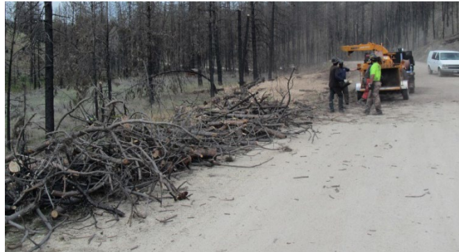
Figure 6.a.3. Chipping can provide a means of slash disposal that reduces smoke emissions and can support soil health. Chipping is typically not an option for burnt material due to the heavy wear inflicted on the machinery.
