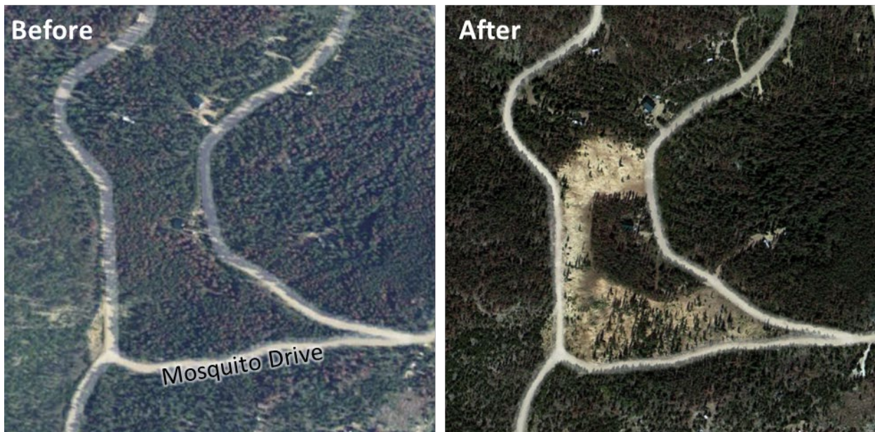
Figure 6.a.2. Effective roadside fuel treatments remove enough trees to result in widely-spaced crowns, remove ladder fuels (seedlings, saplings, shrubs, and low limbs), and reduce surface fuels. More dramatic tree removal along roadways can create even safer roadside conditions where appropriate.
