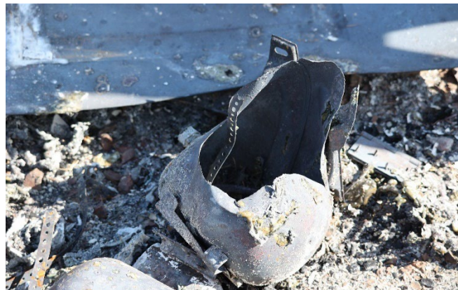
Figure 2.b.8. This propane tank, utilized to fuel a grill, was exposed to high amounts of radiant heat and eventually direct flame contact as the home it was adjacent to burned, causing the gas to ignite and spread the fire further.
