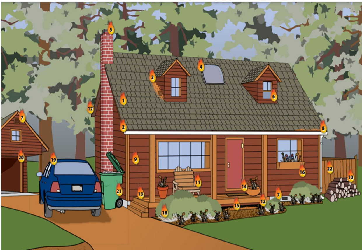
Figure 2.b.9. Common fuel sources and points of ignition around a home. (Source: University of Arizona Extension, nd)
